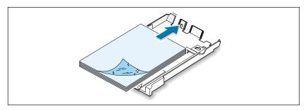
• Load letterhead paper face down with the top of the page going into the tray first.
